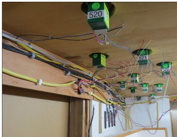
*Track switches in the SLO yard are operated by devices mounted under the layout and accessible from the workshop below. Components are labeled to help find and fix any problem that arises. Wiring is by Tom Machut and Karl Kvilvang.*
