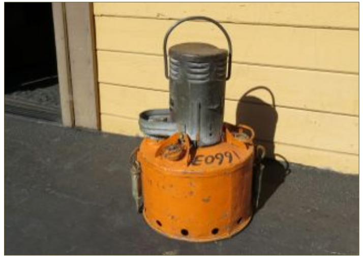
This Preco heater is a rare survivor of Southern Pacific Railroad's ice-bunker refrigerator car era. It's now in the Museum's collection and on display thanks to the efforts of Curator Brad LaRose and regular volunteer Gary See.
